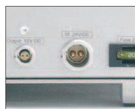
All battery powered instruments have an input range between 18 and 24 V DC
